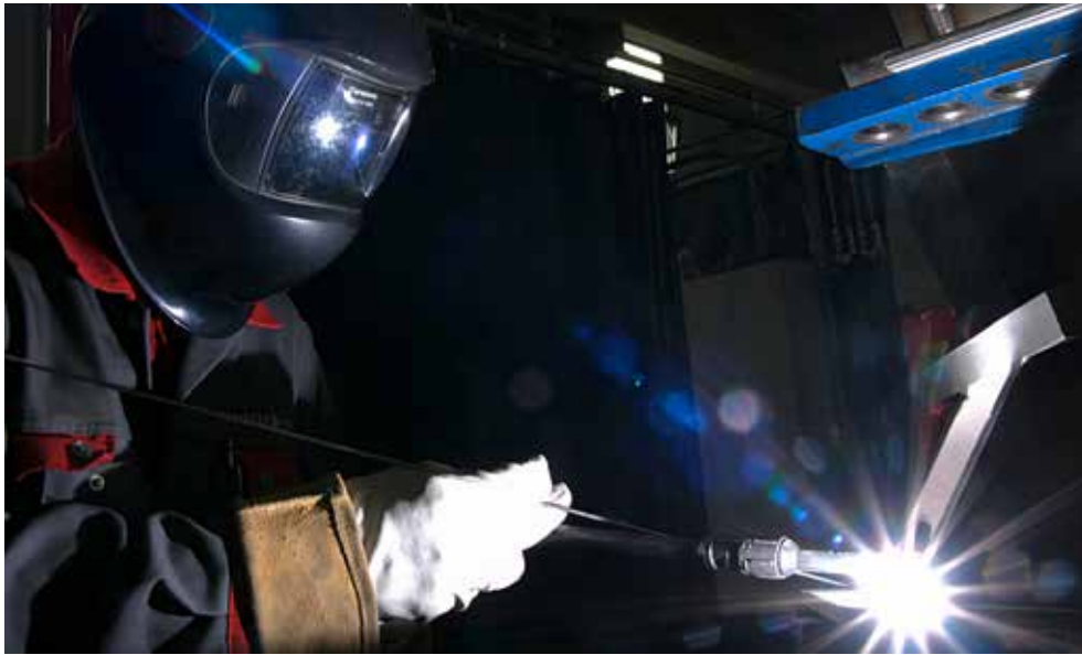
Welding of a vacuum component
