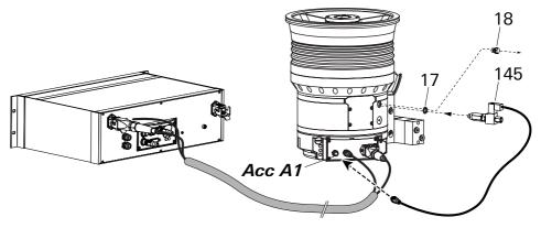
Fig. 12: Connecting the sealing gas valve
