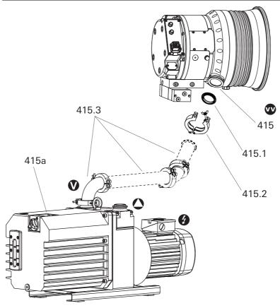
Fig. 8: Connecting the backing pump
