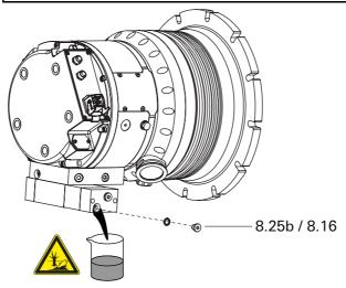
Fig. 14: Draining the operating fluid
