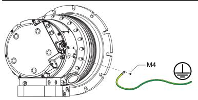
Fig. 9: Installing the earthing connection
