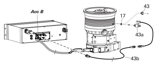
Fig. 13: Connecting the venting valve
