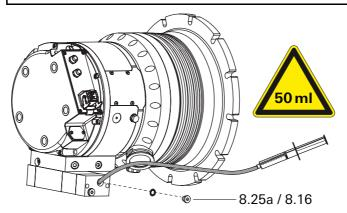
Fig. 7: Filling up the operating fluid
