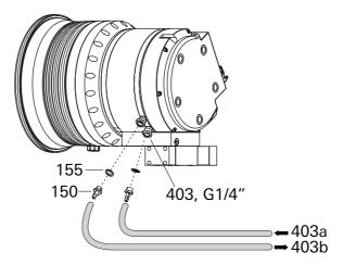
Fig. 11: Connecting the cooling water
