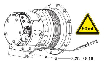
Fig. 15: Filling up the operating fluid
