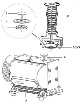
Fig. 8: Replacing the diaphragms
