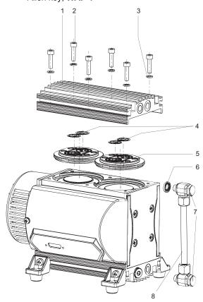
Fig. 7: Pump head and valves
