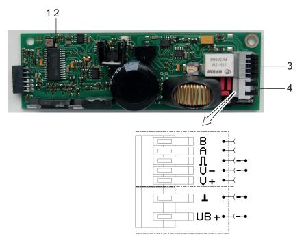
Fig. 4: Circuit board with terminals
