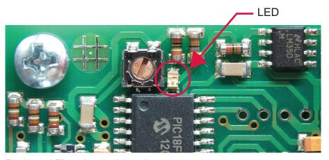
Fig. 10: LED on the circuit board
