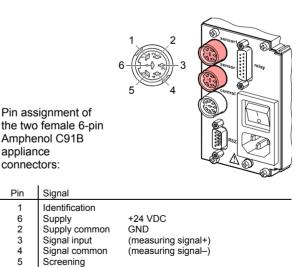
**3.5** *control* **Connector** This connector allows to read the measuring signal, to evaluate the state of the floating contacts of the error relay, and to activate or deactivate the gauges ( $\rightarrow \square 48$ ).
