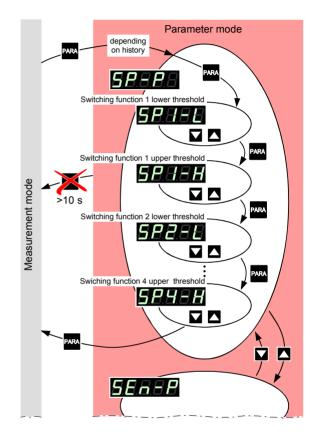
The TPG 262 has four switching functions with two adjustable thresholds each. The status of the switching function is displayed on the front panel ( $\rightarrow$  24, 21) and can be evaluated via the floating contacts at the *Control* connector.
