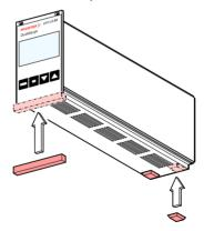
... and slip the supplied rubber bar onto the bottom edge of the front panel.
