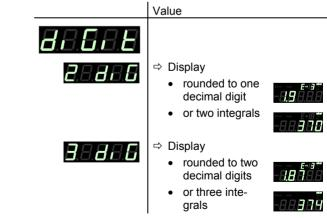
When the PrE ( $\rightarrow$   $\square$  47) is ON and the pressure is in the range p<1.0E-4 mbar the display resolution of the PCR Gauge is reduced by one decimal digit.
