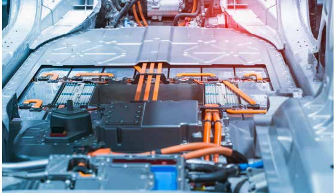
Battery pack with cooling system
