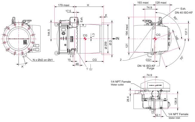
Fig. 7: Dimensions ATP 1603 M with OBC
