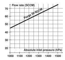
Fig. 6: Purge flow diagram
