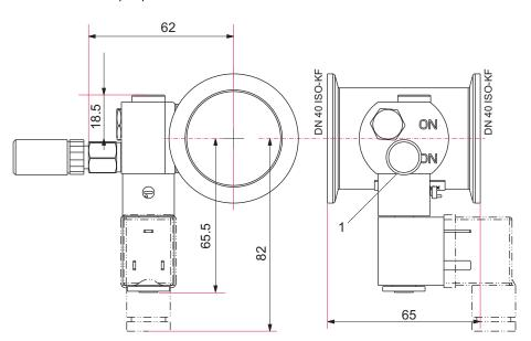
Fig. 9: Dimensions of Air inlet solenoid valve
