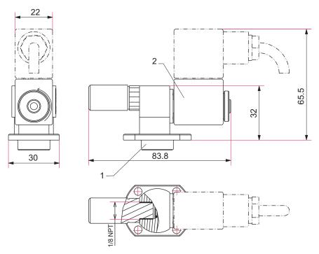
Fig. 8: Dimensions of Purge solenoid valve
