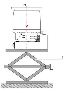
Fig. 5: Installing the pump inlet facing up
