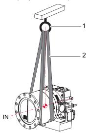
Fig. 4: Horizontal pump installation
