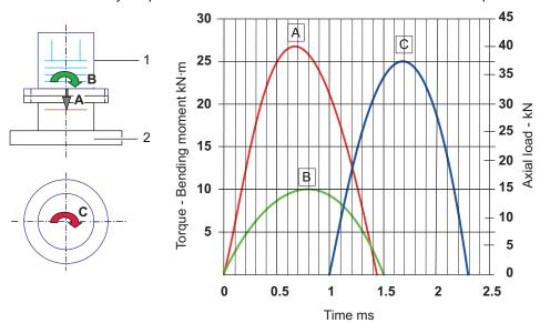
Fig. 2: Graph of the loads exerted on the equipment
