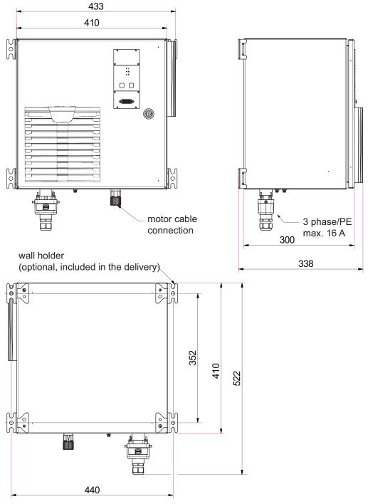
Fig. 22: Electronic drive unit RC 5500 Dimensions in mm
