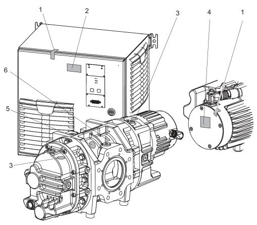
Position of stickers on product with horizontal direction of flow Fig. 3:
