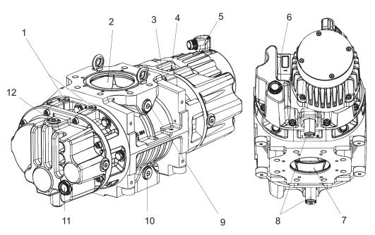
Fig. 5: Design, HiLobe for vertical direction of flow
