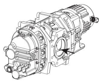
Fig. 10: Mounting orientation: Horizontal direction of flow
