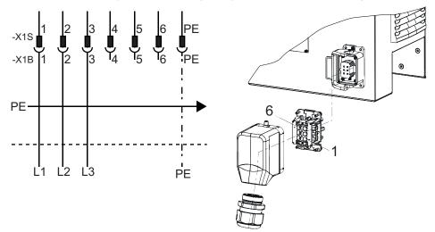
Fig. 14: Mains connection pin assignment
