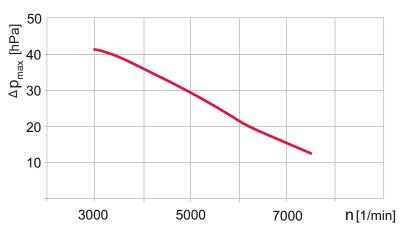
Fig. 4: Permissible pressure differential between input and output sides, as a function of pump rotation speed
