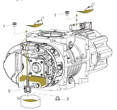
Fig. 19: **Filling with lubricant**
