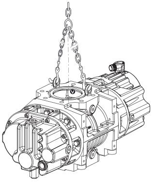
Fig. 8: Transporting vacuum pump
