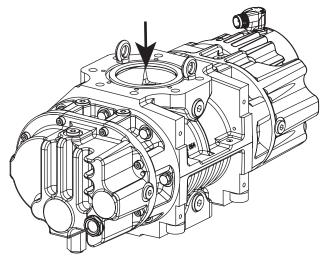
Fig. 9: Mounting orientation: Vertical direction of flow
