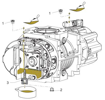
Fig. 11: Filling with lubricant
