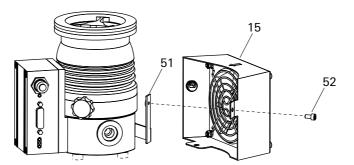
$\rightarrow$  Fix fan housing 15 with Allen head screw 52 at mounting bracket.
