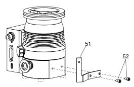
→ Fix mounting bracket 51 with two Allen head screws 52 at the pump bottom part.
