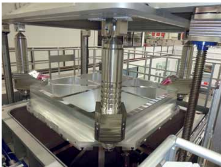
Figure 3: Work pieces are transported into the chamber with special lifting gear
