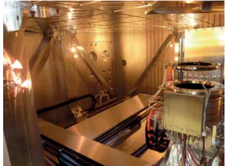
Figure 2: Using a three-axis manipulator system inside the chamber of the IBF-2000, work pieces with a diameter up to 2,000 mm can be processed
