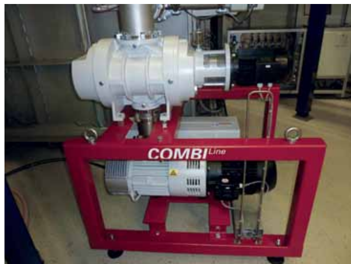
Figure 5: The Pfeiffer Vacuum CombiLine pumping station inside the IBF-2000
