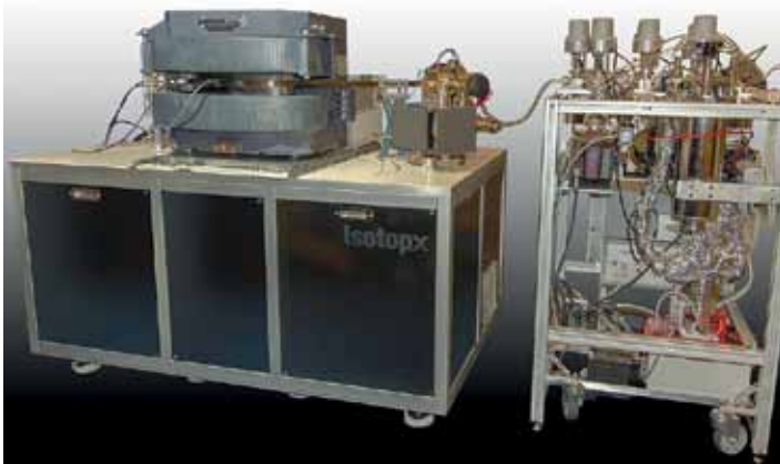
Figure 1: Noble gas mass spectrometer with attached ultra high vacuum sample preparation system using the Pfeiffer Vacuum HiCube pumping system
