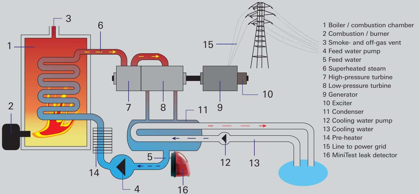
The condenser is the interface between the closed water-steam-circuit, the steam turbine and the cooling circuit. The water vapor condenses on pipes filled with coolant water, and is then available for steam generation again.
