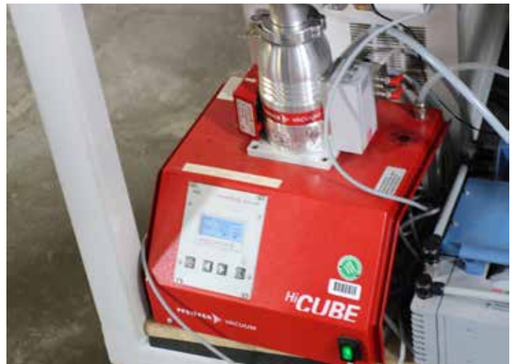
Figure 7: The turbopumping station sponsored by Pfeiffer Vacuum shown in action.
