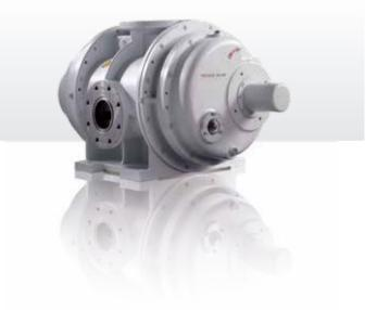
In addition to traditional Roots pumps, there are also gascirculation-cooled pumps (OktaLine G). Instead of an overflow valve, the pump has gas-circulation cooling. The gas flows from the outlet flange, is cooled in a heat exchanger and is
