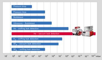
Leak rates in the range of below  $10^{-6}$  mbar l/s can only be determined with certainty using the helium leak detector.
