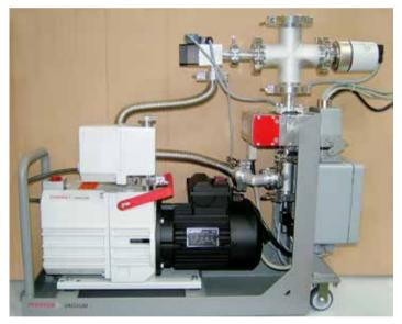
Figure 1: customized pumping cart for solar receiver degassing
