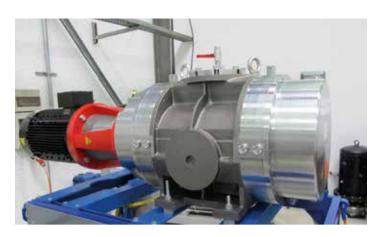
Tritium compatible Roots pump Okta 1500 GM with highest compression for hydrogen
