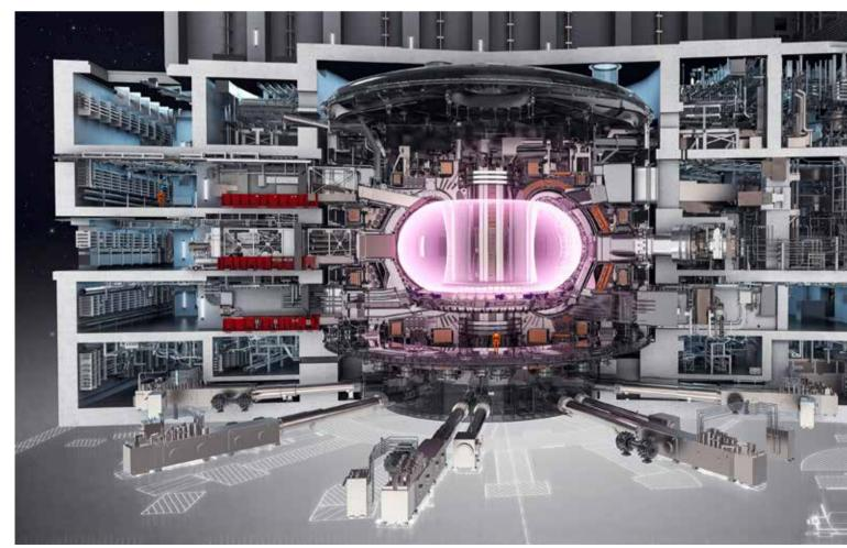
The opposite applies to the material used to manufacture the vacuum recipient. Here, the highest possible magnetic permeability is required. This means that the externally induced magnetic fields should not be deflected and the material should not be heated by eddy currents.
