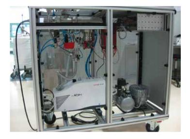
Special leak detector for a very wide range of applications. All gases from  $H_2$  to Xe can be detected within a wide pressure
