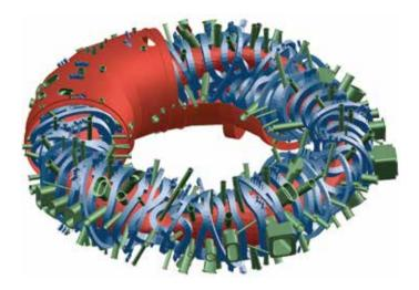
Computer graphic: Cryostat, magnetic coils and plasma vessel at Wendelstein 7-X fusion reactor (image: IPP)
