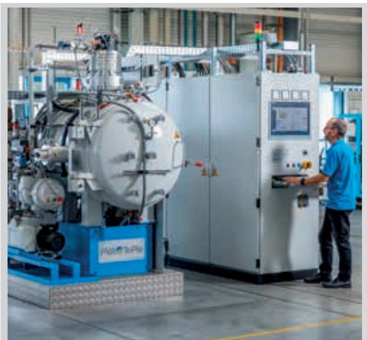
Vacuum soldering furnaces built by PVA TePla Courtesy of PVA TePla
