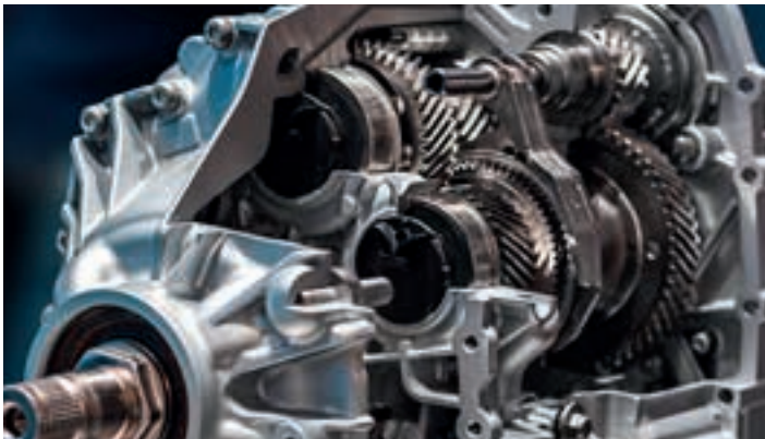
Gears hardened under vacuum
