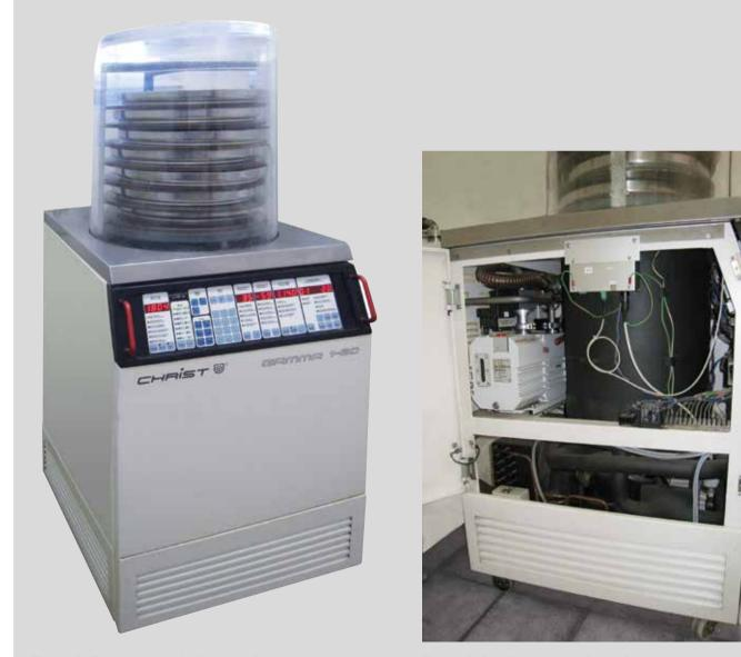
Figure 2: Freeze-drying facilities on Becker's Mare's Milk Farm
