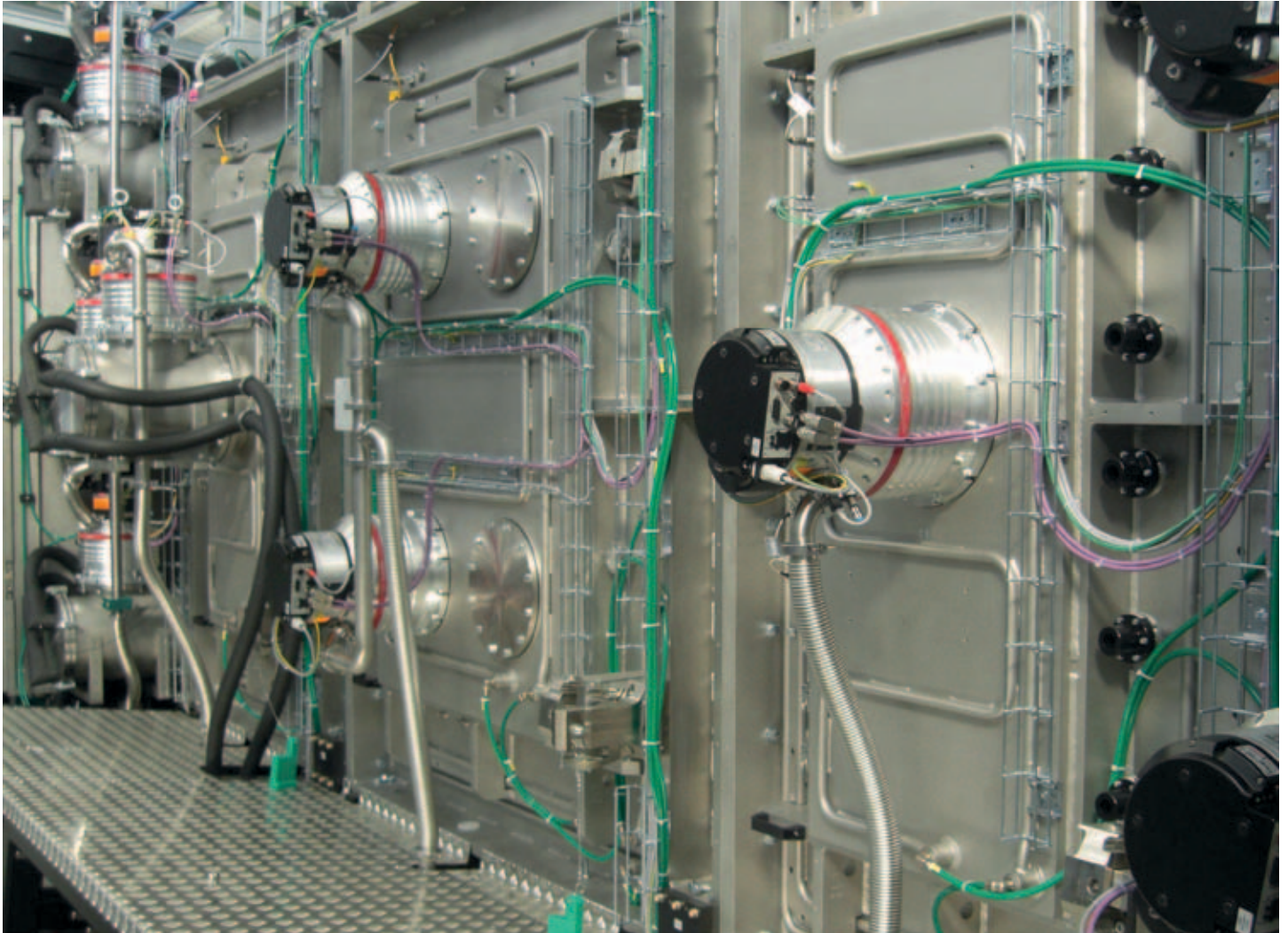
Figure 2: Glass coater of Leybold Optics with HiPace turbopumps by Pfeiffer Vacuum
