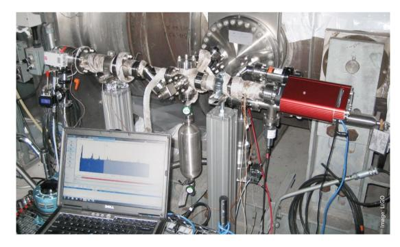
Fig. 3: The vacuum solutions of Pfeiffer Vacuum used at the LIGO experiment – HiPace turbopump and Prisma Plus mass spectrometer
