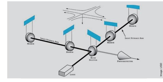
Fig. 2: Scheme of the LIGO interferometer for the detection of gravitational waves
