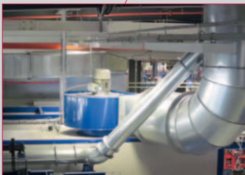
Figure 2: Filtration unit for sorting and recycling coolants, chips and production residues
