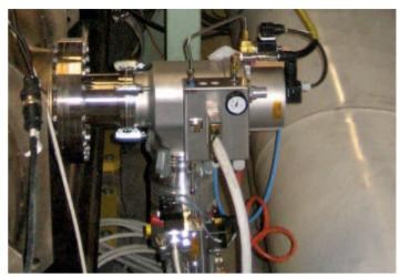
Beam vacuum generation with HiPace 300 turbopump
