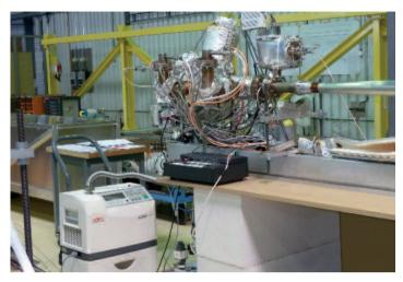
Leak testing system for LHC components with ASM Graph
