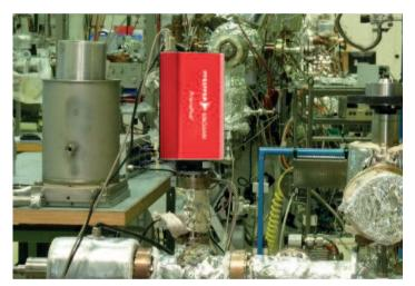
Testing system for the outgassing behavior of LHC components with PrismaPlus
