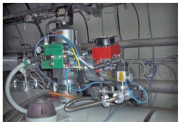
Insulation vacuum generation with HiPace 300 turbopump
