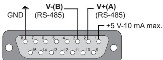
**Fig. 6: Male 15-pin RS-485 connector**
