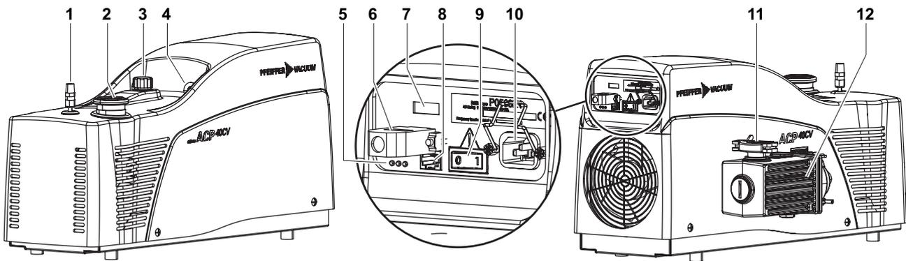
**Fig. 2: ACP 28 - 40 - CV version with single-phase frequency converter**
