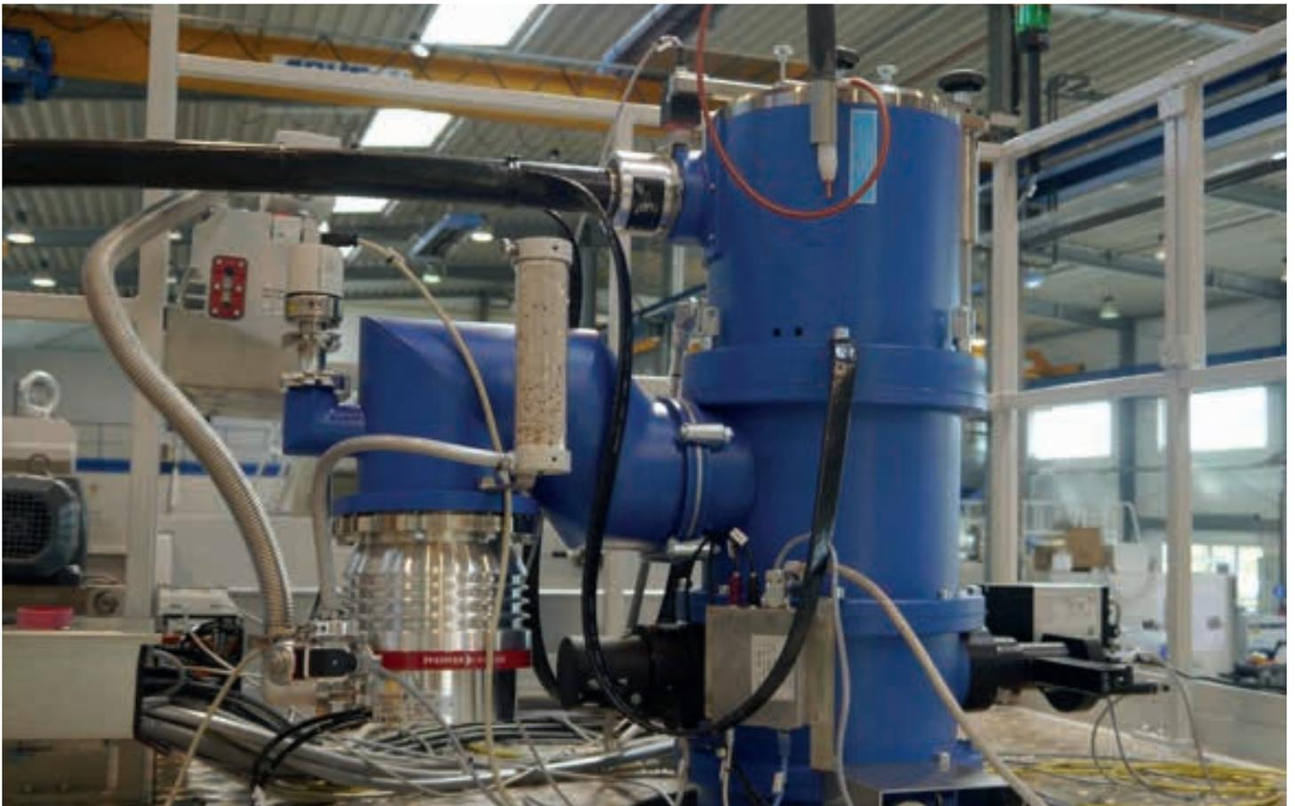
Figure 5: HiPace turbomolecular pump on the electron beam generator
