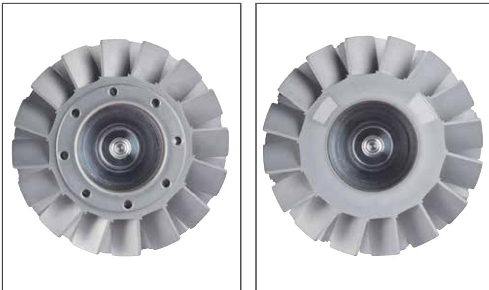
Figure 3: Comparison of a balancing level of conventional balancing (left) with balancing holes and of laser balancing (right) with laser ablation segments
