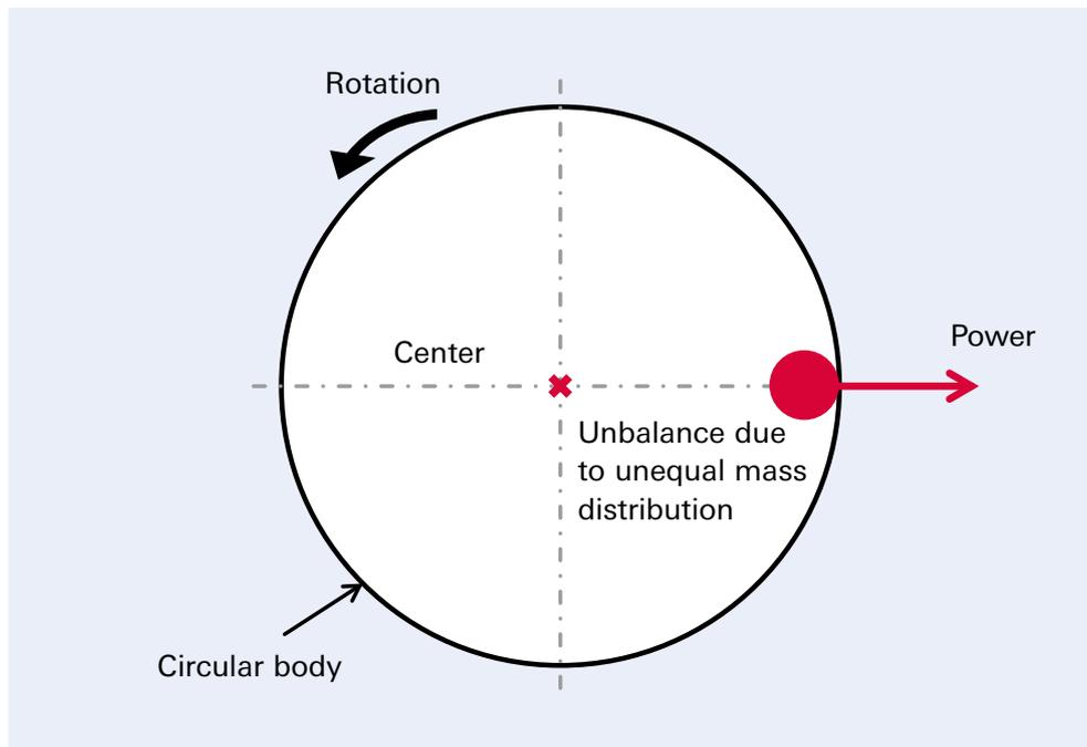
Figure 1: An outwardly symmetrical circular body exhibits unbalance due to unequal mass distribution. The rotation of the body around its center point generates a circulating force, which leads to vibrations.
