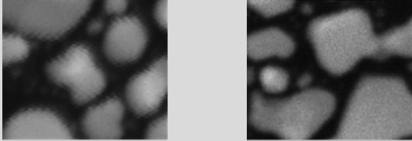
Stronger vibrations (~20 nm) at the high-vacuum flange result in a blurred image at high magnifications.
