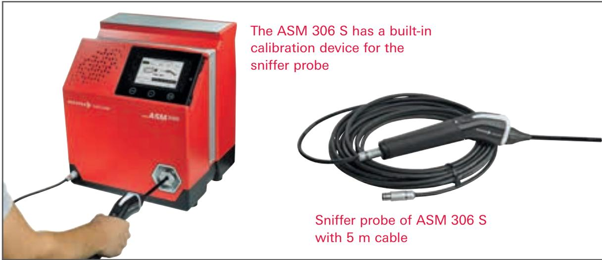
The ASM 306 S has a built-in calibration device for the sniffer probe
