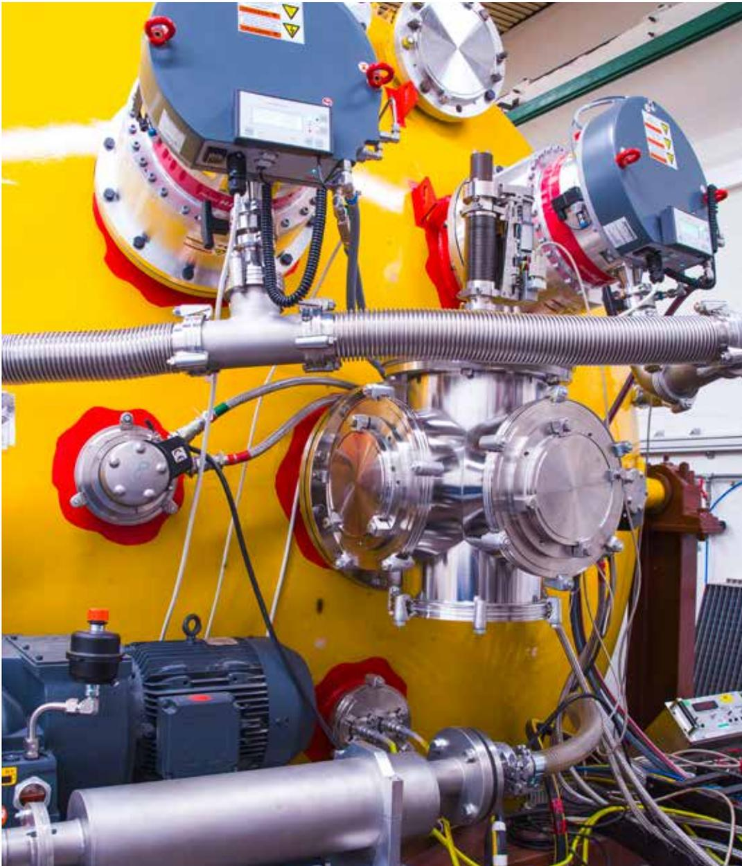
Figure 2: Two ATH 3204 M turbopumps with a Hepta Dry 200 screw pump as a backing pump at the JUMBO space simulation facility for testing ion thrusters. In combination with two HiPace 2300 with Duo 65 backing pumps and eight cryo pumps, a pumping speed of 150,000 liters of Xe per second is achieved.
