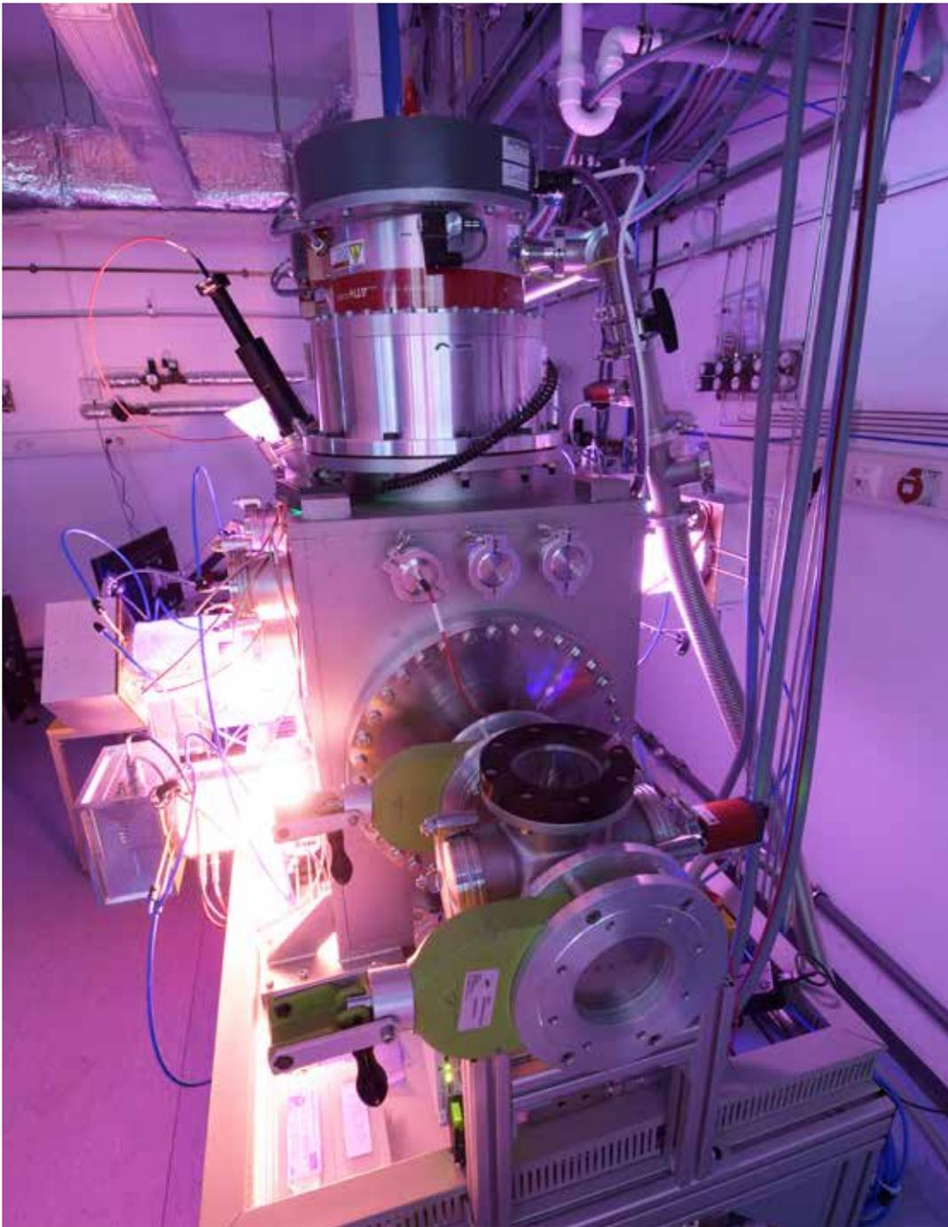
Figure 3: 2DIBS facility with several RF ion sources for coating substrates on both sides using ion beam sputter deposition. This system is also equipped with two turbopumps of the type ATH3204M with ACP 28 backing pumps.
