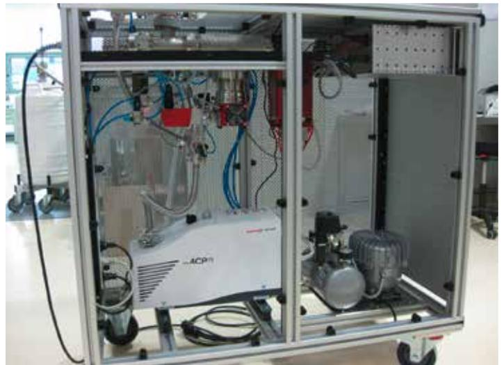
Special leak detector for a very wide range of applications. All gases from H<sub>2</sub> to Xe can be detected within a wide pressure
