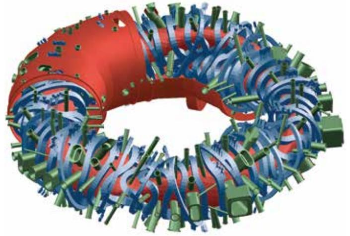
Computer graphic: Cryostat, magnetic coils and plasma vessel at Wendelstein 7-X fusion reactor (image: IPP)
