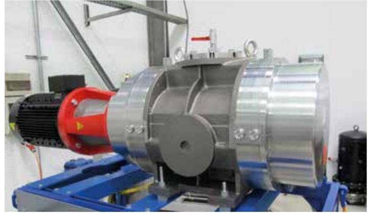
Tritium compatible Roots pump Okta 1500 GM with highest compression for hydrogen
