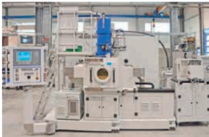
Figure 1: Electron beam welding machine with welding chamber and electron beam generator (courtesy of Steigerwald Strahltechnik)
