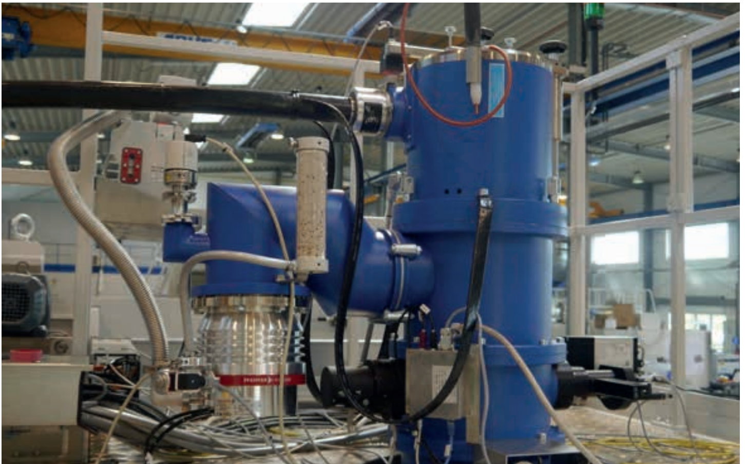
Figure 5: HiPace turbomolecular pump on the electron beam generator Courtesy of Steigerwald Strahltechnik
