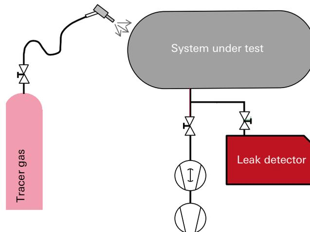
A further method is the sniffing test. Here, the system is pressurized with a tracer gas such as helium. A sniffer probe is then passed over the system. In the event of a leak, the leak detector discovers the escaping tracer gas and thereby localizes the leak. Since helium is usually added during the EBM process, anyways, this method can also be used to guarantee a helium supply.
