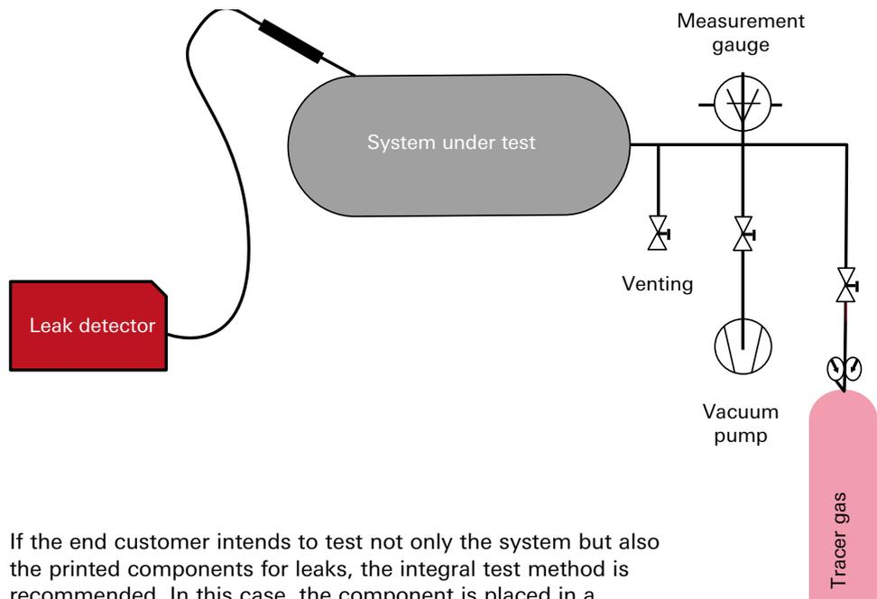
If the end customer intends to test not only the system but also the printed components for leaks, the integral test method is recommended. In this case, the component is placed in a vacuum test chamber and filled with tracer gas. If there is a leak, the tracer gas will escape from the component into the test chamber and will be measured by the leak detector.
