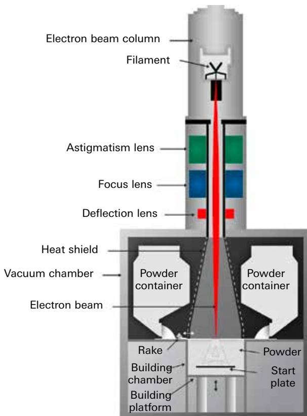
Figure 2: Arcam EBM system, schematic representation
