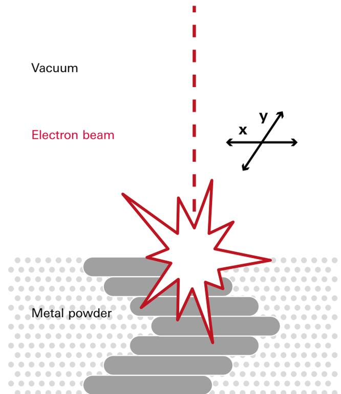
Figure 3: Melting of the metal powder layer by layer
