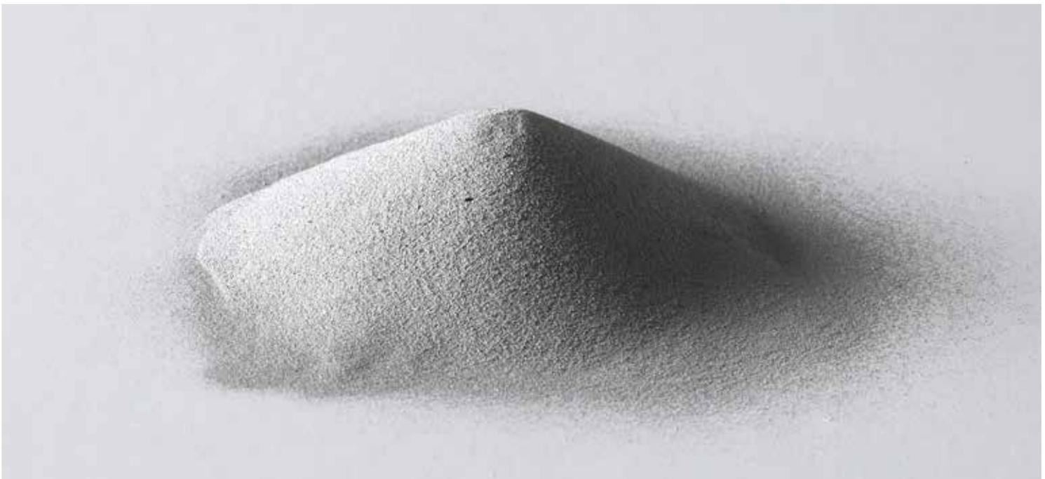
Figure 4: Metal powder for 3D printing; alloys of titanium and cobalt-chrome are often used
