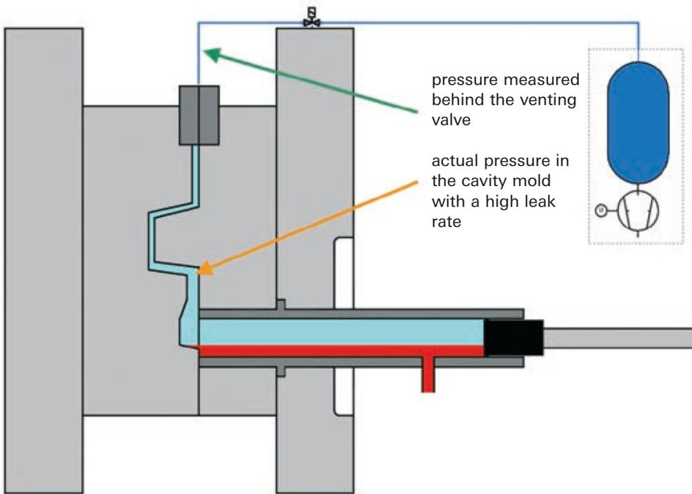
Figure 1b: Vacuum process with metal dosing during the evacuation process
