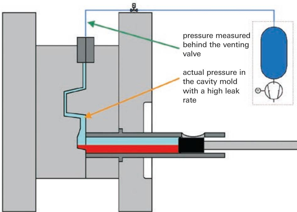
Figure 1a: Standard vacuum process for pressure die-casting
