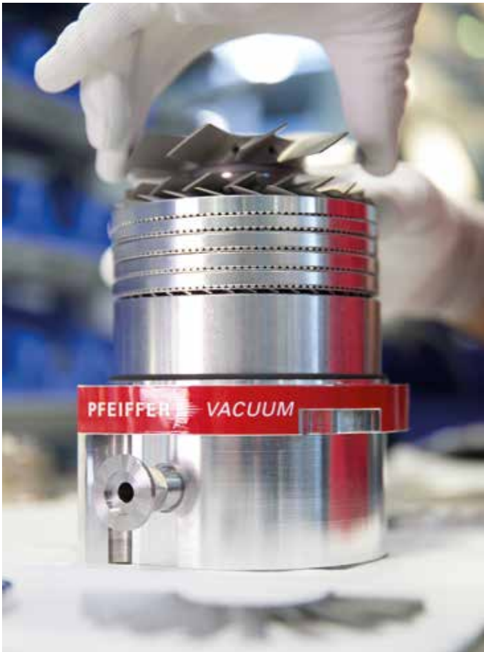
Figure 2: Turbopump rotor replacement
