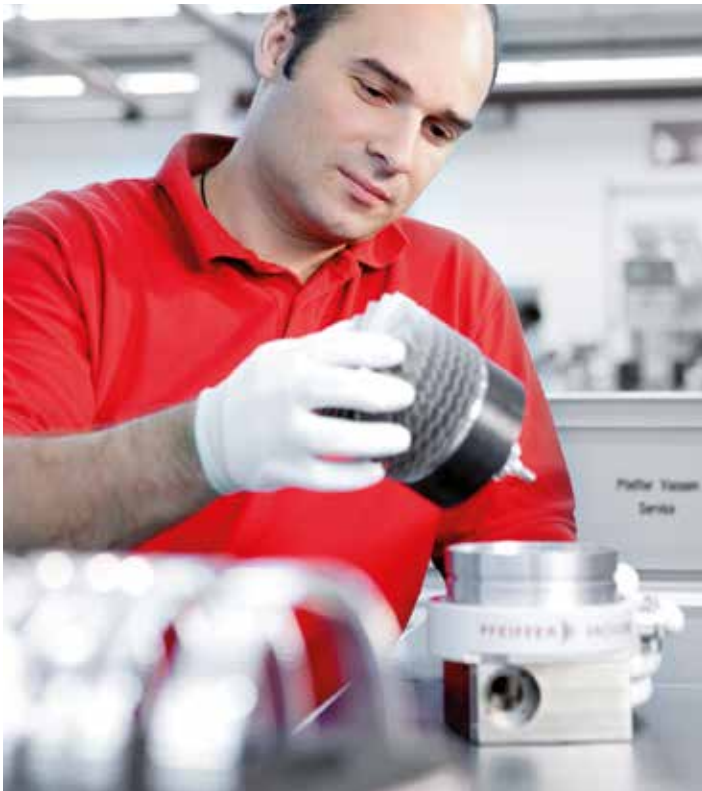
Figure 8: Service of a turbopump
