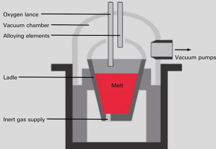
Figure 1: VOD (Vacuum-Oxygen-Decarburisation) Process
