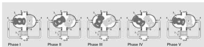
Figure 5: Operating principle of a gas-cooled Roots pump
