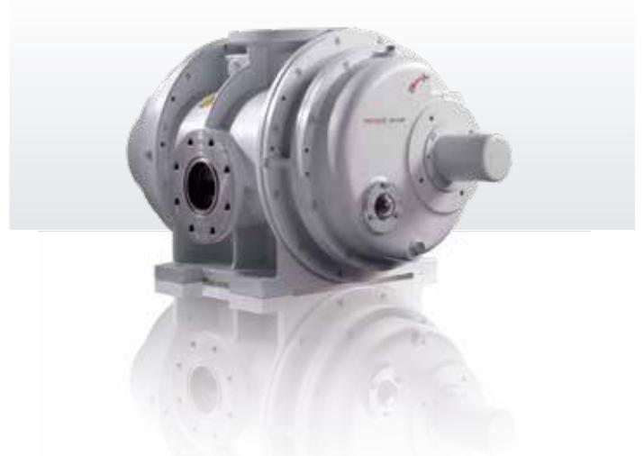
In addition to traditional Roots pumps, there are also gas-circulation-cooled pumps (OktaLine G). Instead of an overflow valve, the pump has gas-circulation cooling. The gas flows from the outlet flange, is cooled in a heat exchanger and is
