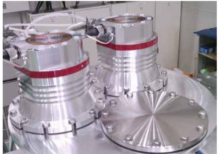
Images 3 and 4: HiPace turbopumps installed at European XFEL
