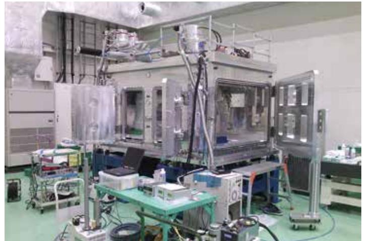
Image 6: Interaction chamber at European XFEL equipped with Pfeiffer Vacuum solutions (© European XFEL)
