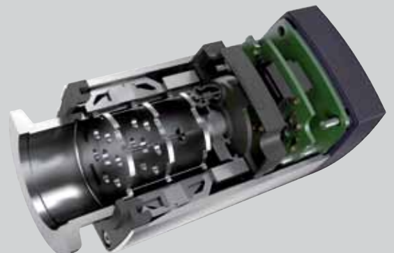
Cross section of the IKT sensor
