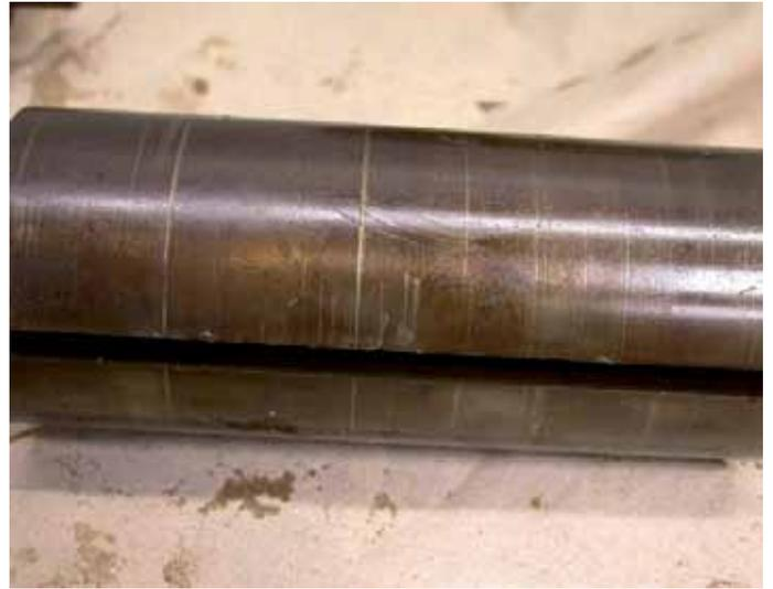
Figure 3 and 4: Inlet port of a rotary vane pump without a dust filter. Rotor was tarnished in the cylinder. Pump system must be replaced.
