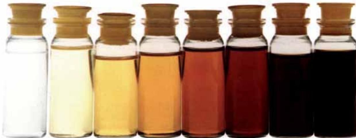
Figure 2: Color scale of the fluid aging of mineral oil.
