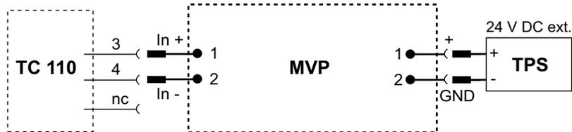
Fig. 5: Connection to TC and TPS
