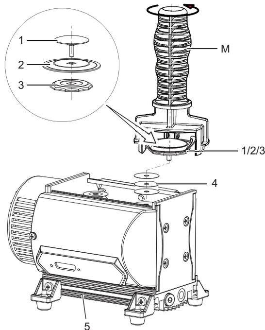
**Fig. 8: Replacing the diaphragms**
