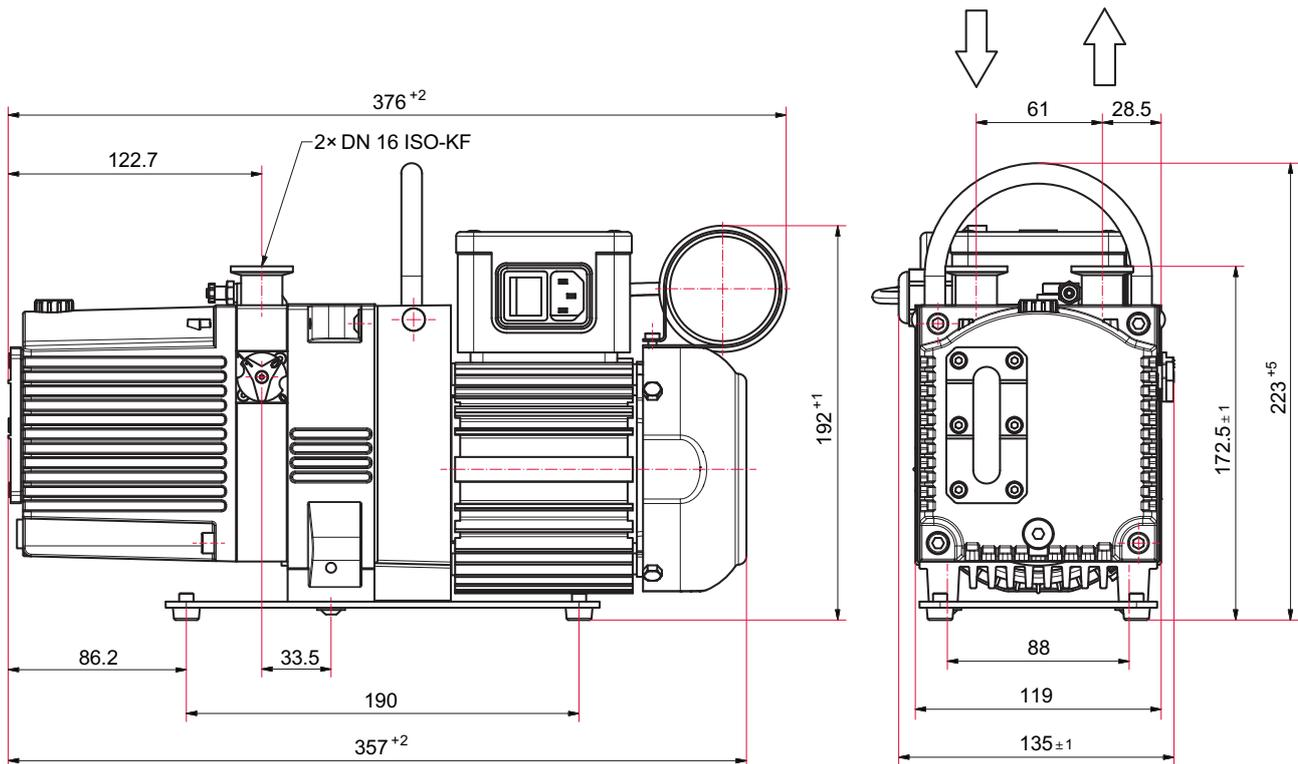
Fig. 21: Dimensions Duo 1.6 M, 100 V, 50 Hz with switch, 95-105 V, 60 Hz
