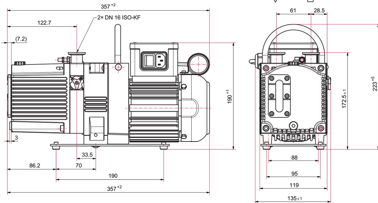
Fig. 23: Dimensions Duo 1.6 M, single-phase motor, 230-240 V, 50/60 Hz
