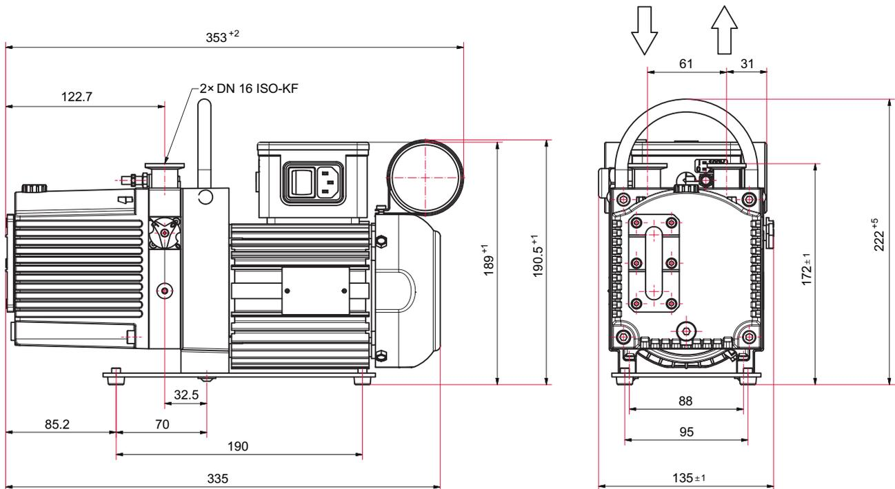
Fig. 18: Dimensions Duo 1.6, single-phase motor, 100/200 V, 50/60 Hz
