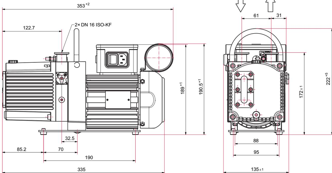
Fig. 19: Dimensions Duo 1.6, single-phase motor, 115/230 V, 50/60 Hz
