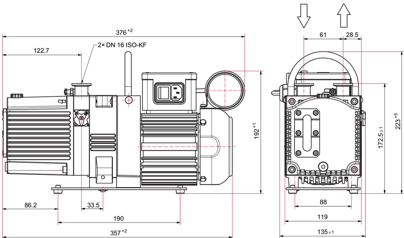
Fig. 22: Dimensions Duo 1.6 M, single-phase motor, 105 V, 50 Hz | 115-125 V, 60 Hz
