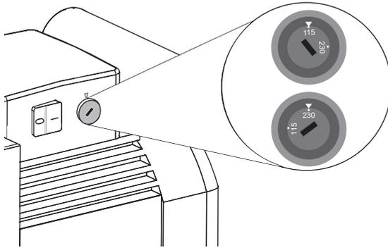
**Fig. 9: Voltage selector switch on the terminal box**
