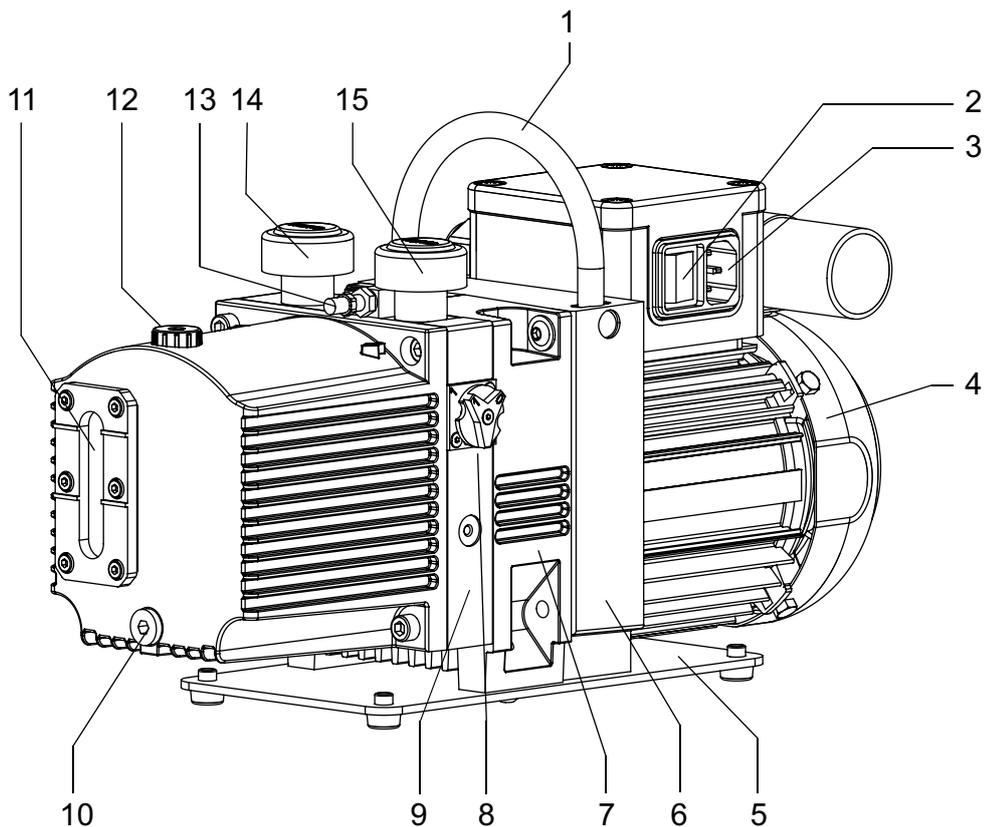
**Fig. 2: Structure of the rotary vane pump**
