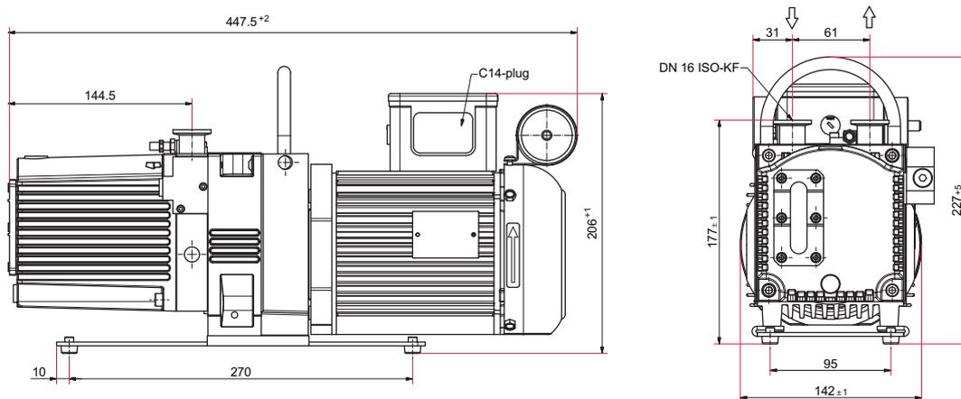
Fig. 21: Dimensions Duo 6 MC - 115/230 V, 50/60 Hz, switchable
