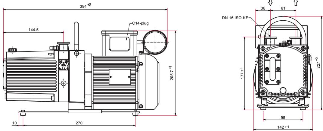
Fig. 18: Dimensions Duo 6 - 100 - 115 V, 50/60 Hz
