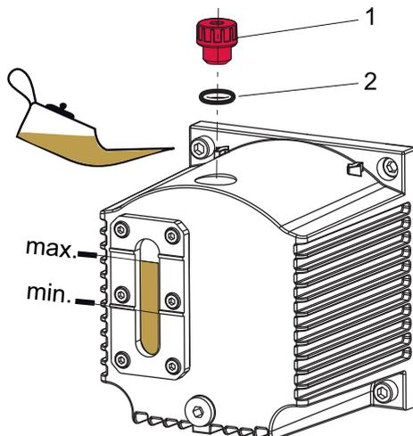
**Fig. 10: Filling the operating fluid**
