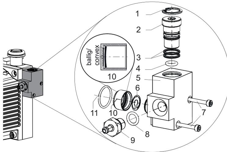
**Fig. 16: Gas ballast valve with flushing gas connection**
