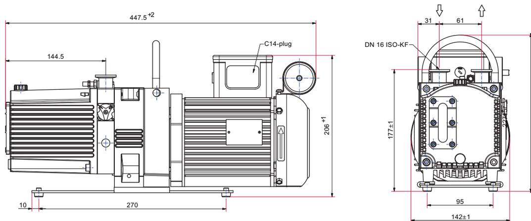
Fig. 19: Dimensions Duo 6 M - 115/230 V, 50/60 Hz, switchable
