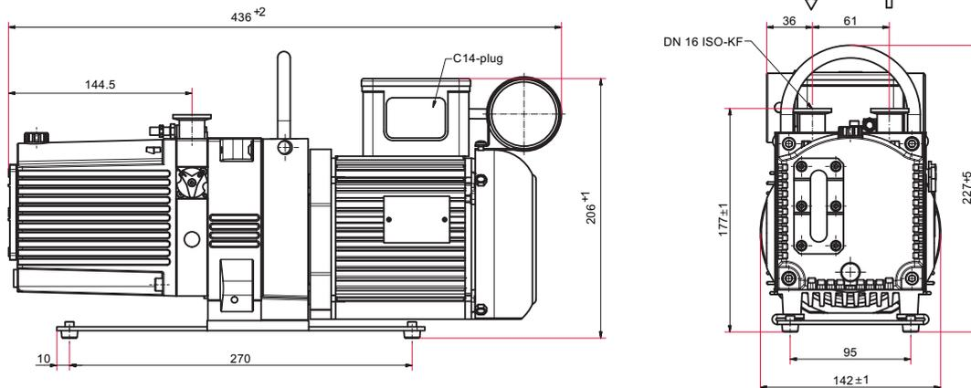
Fig. 20: Dimensions Duo 6 M - 100 – 115 V, 50/60 Hz
