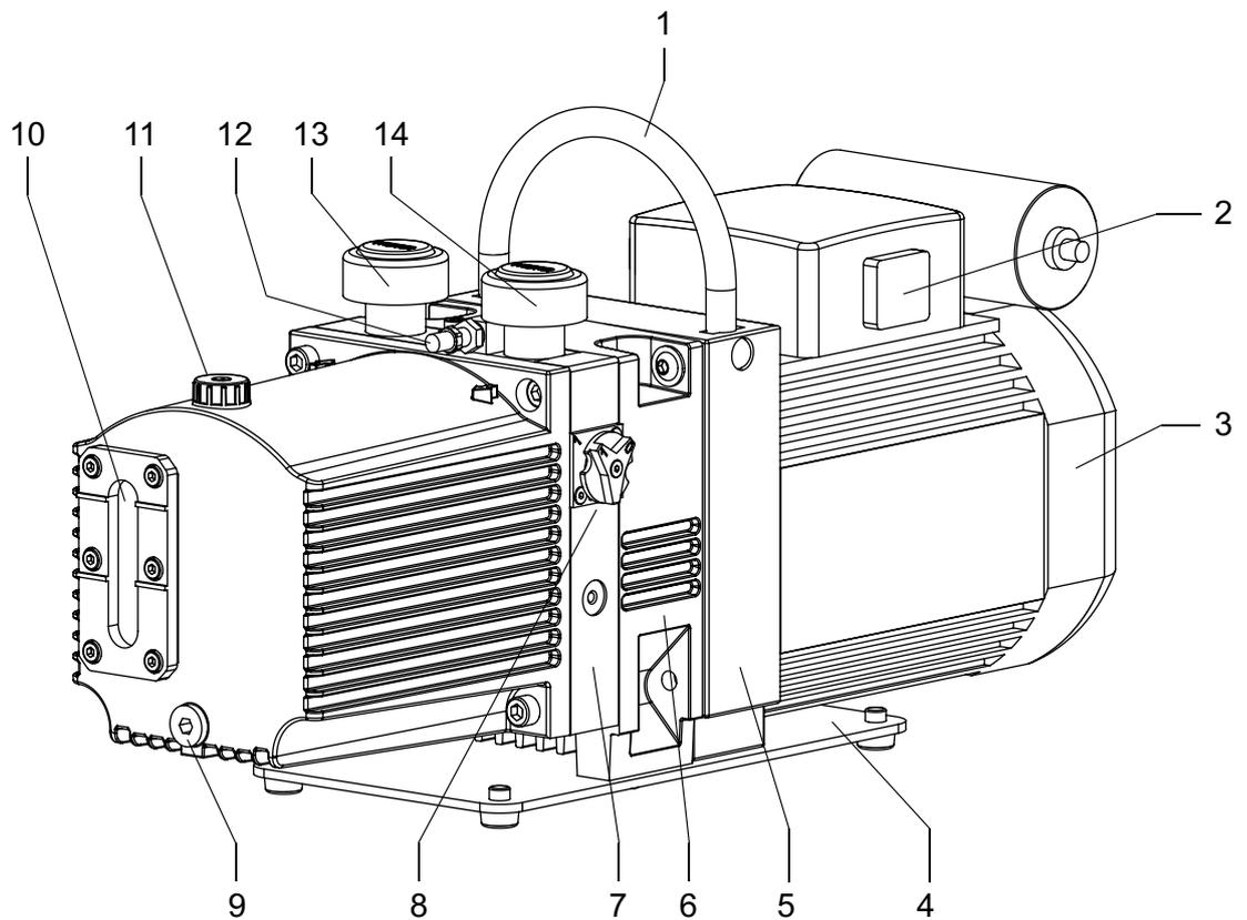
Fig. 2: Structure of the rotary vane pump
