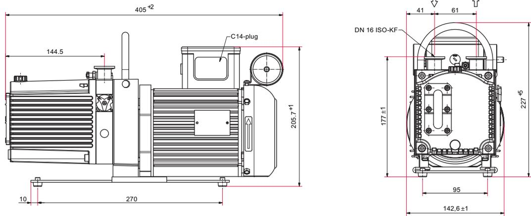
Fig. 17: Dimensions Duo 6 - 115/230 V, 50/60 Hz, switchable
