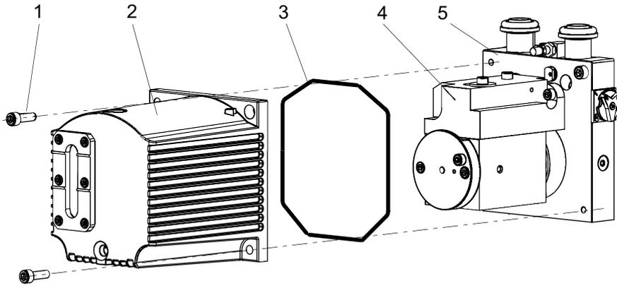
**Fig. 14: Remove/fit rotary vane vacuum pump cap**
