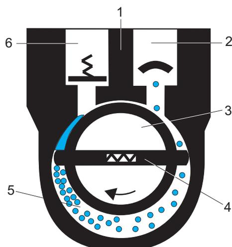
**Fig. 3: Rotary vane vacuum pump functional principle**
