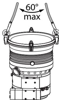
Fig. 1: Transport in valid orientation
