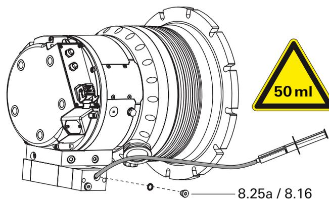
**Fig. 15: Filling up the operating fluid**
