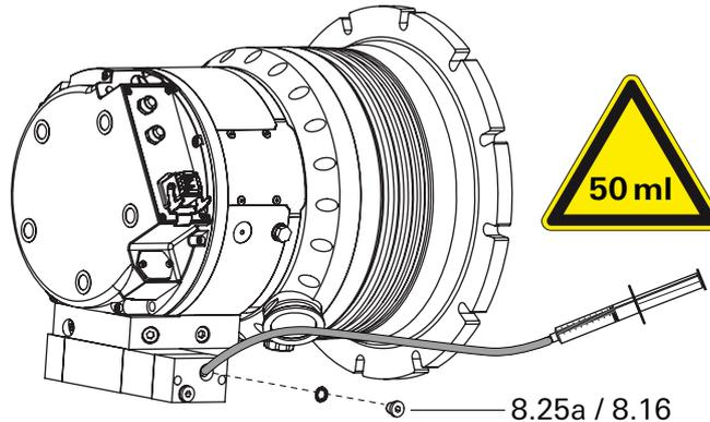
Fig. 7: Filling up the operating fluid
