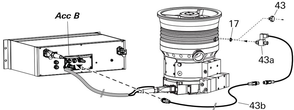
**Fig. 13: Connecting the venting valve**
