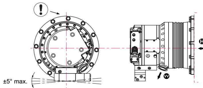
Fig. 6: Admissible fixing and the position of the operating fluid pump for horizontal installation of the turbopump horizontal
