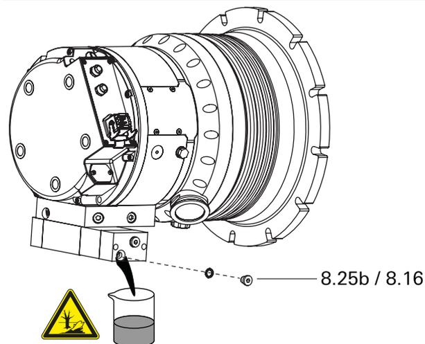
**Fig. 14: Draining the operating fluid**
