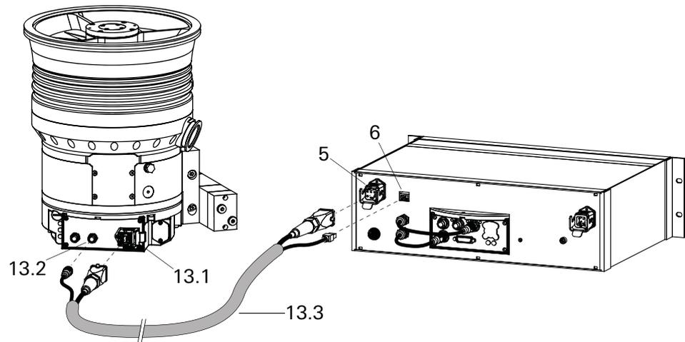
**Fig. 10: Connecting the turbopump to the electronic drive unit TCP 1200**
