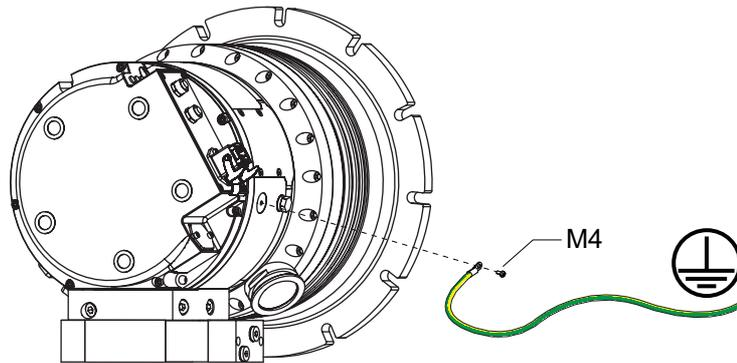
Fig. 9: Installing the earthing connection
