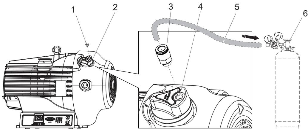
**Fig. 9: Connecting gas ballast external supply**
