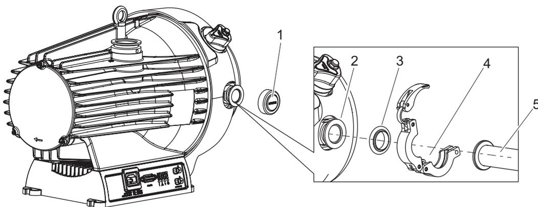
Fig. 8: Example of exhaust connection
