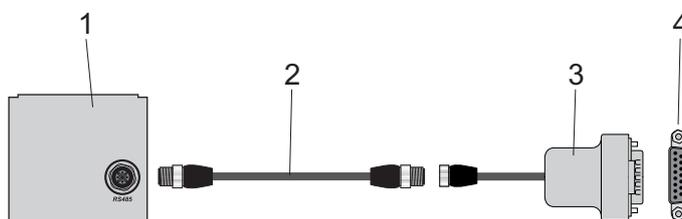
**Fig. 13: Connecting a control unit via the "remote" connection**
