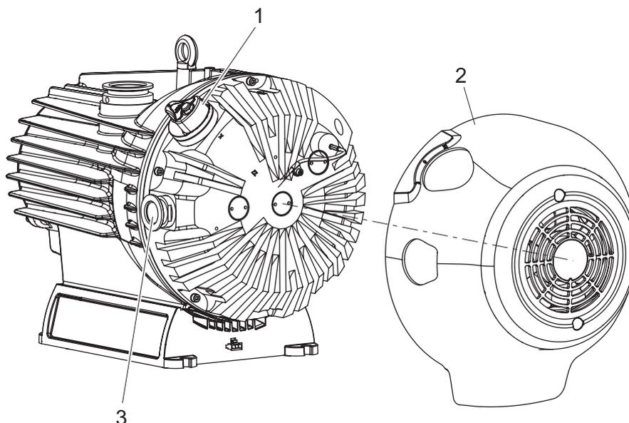
**Fig. 22: Removing fan cover**
