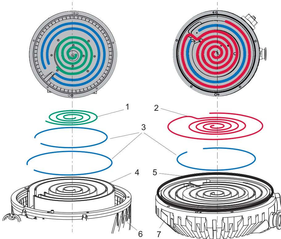
**Fig. 30: Replacing tip seals on scroll pump**
