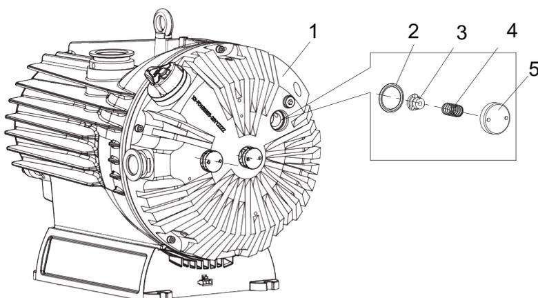
**Fig. 23: Disassembling valves**
