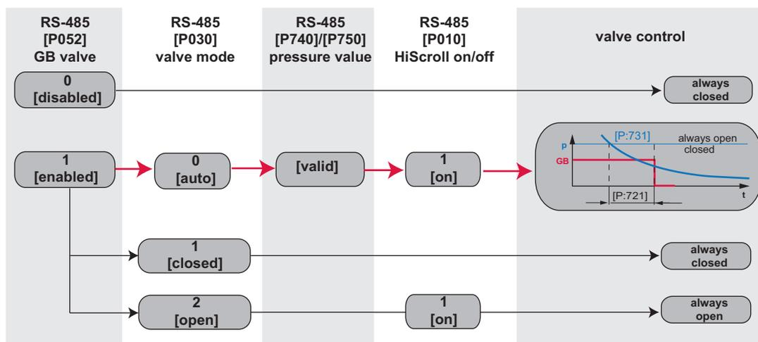
Fig. 18: Pressure-dependent gas ballast valve control in automatic mode
