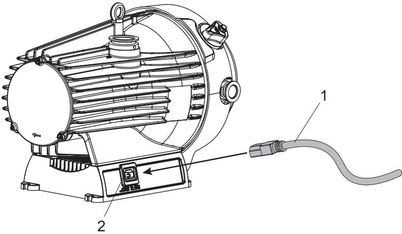
**Fig. 10: Connecting to mains power supply**
