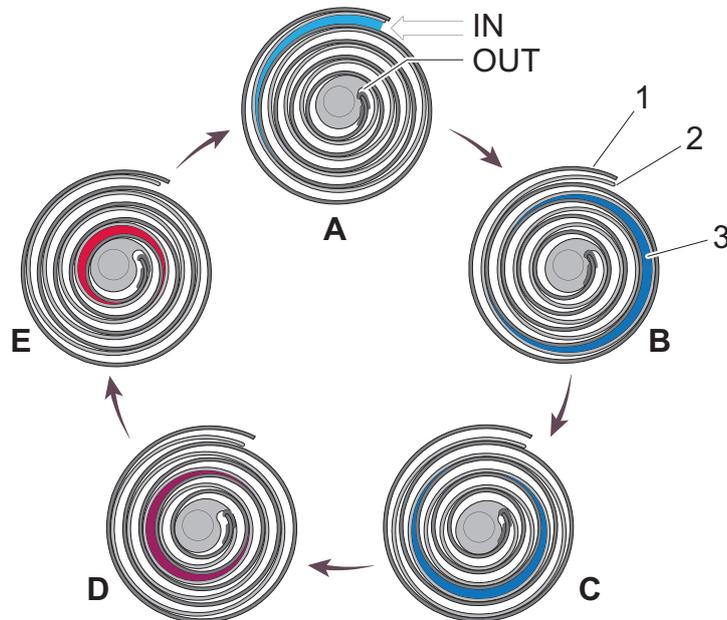
**Fig. 3: Schematic compression cycle of scroll pumps**
