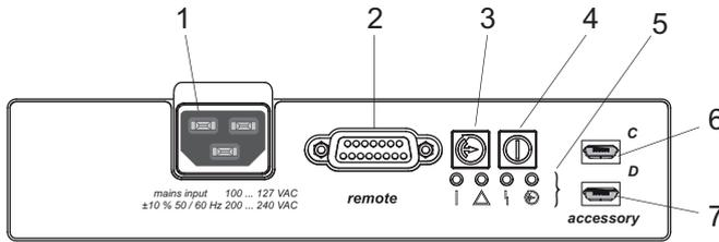
Fig. 11: Interfaces of the electronic drive unit
