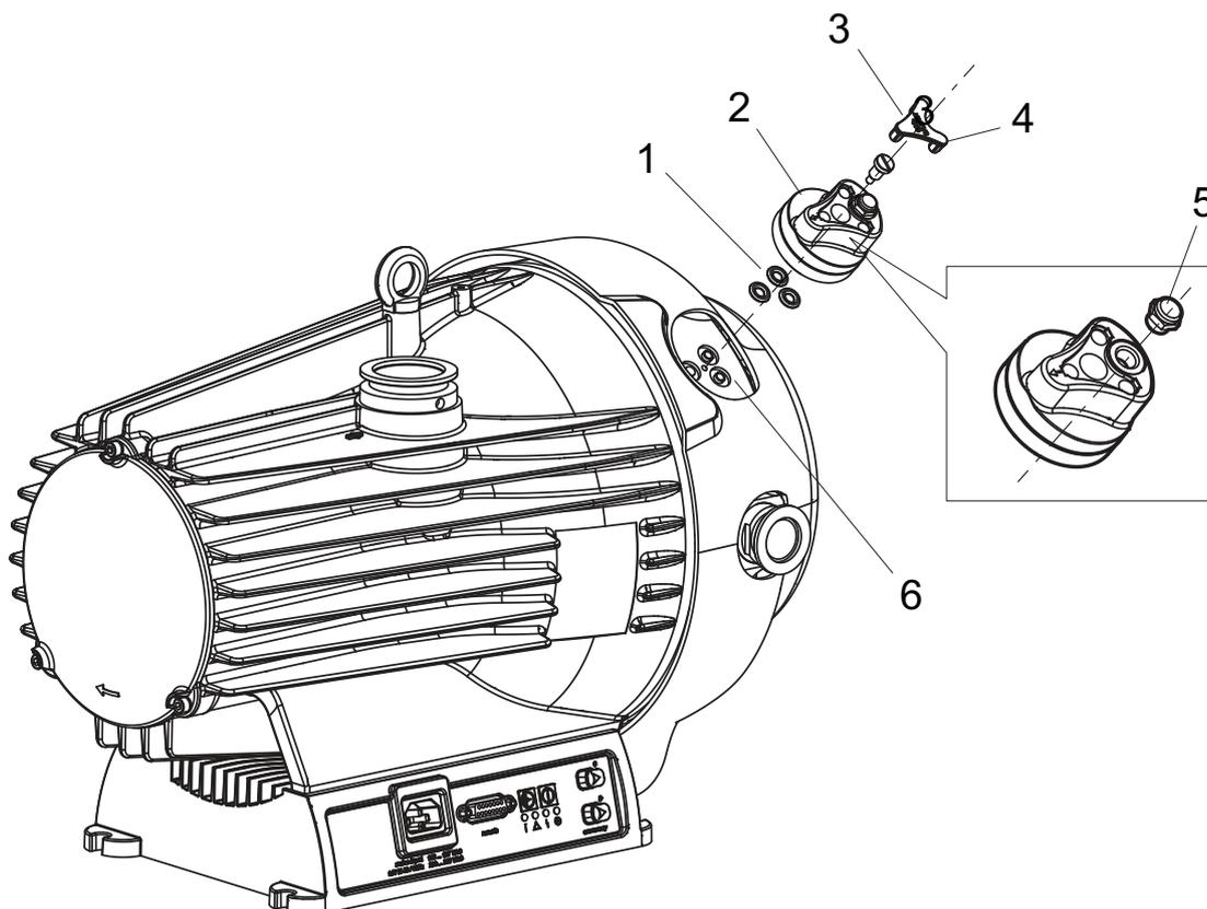
**Fig. 25: Disassembling gas ballast valve**
