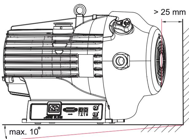
Fig. 6: Minimum distances and permissible inclination
