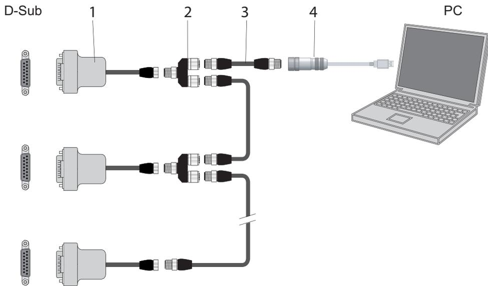
**Fig. 14: Cross-link via connection RS-485 using connection cables and accessories**
