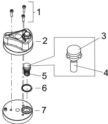
Fig. 27: Assembling gas ballast valve
