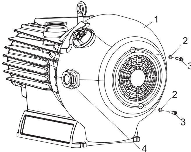
**Fig. 20: Unscrewing and removing cylinder screws**
