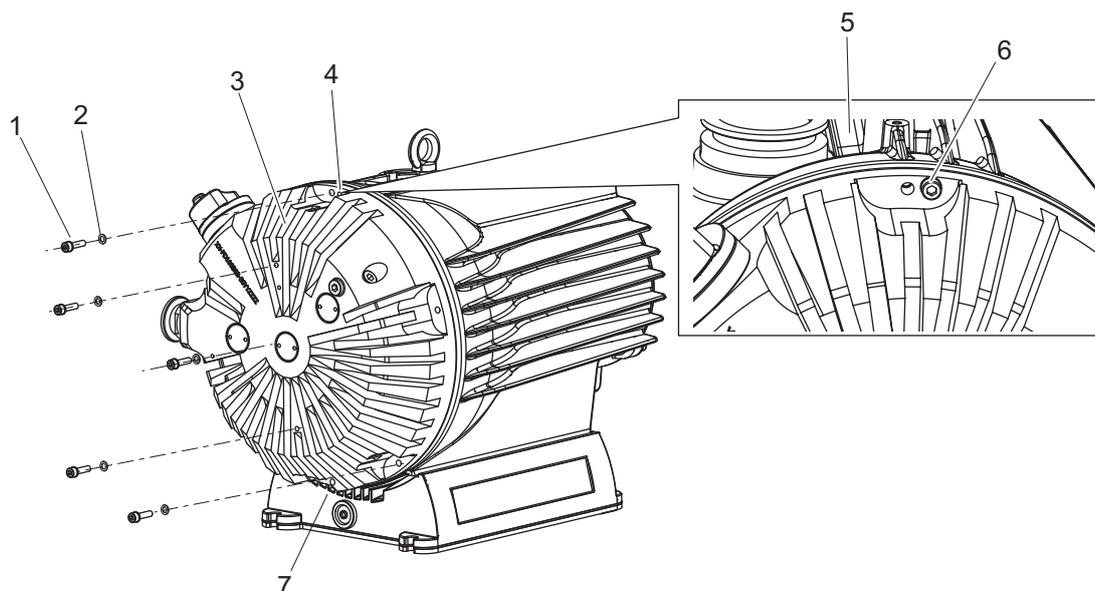
**Fig. 29: Removing the spiral housing**
