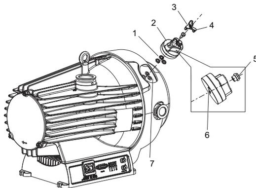
Fig. 28: Assembling gas ballast valve
