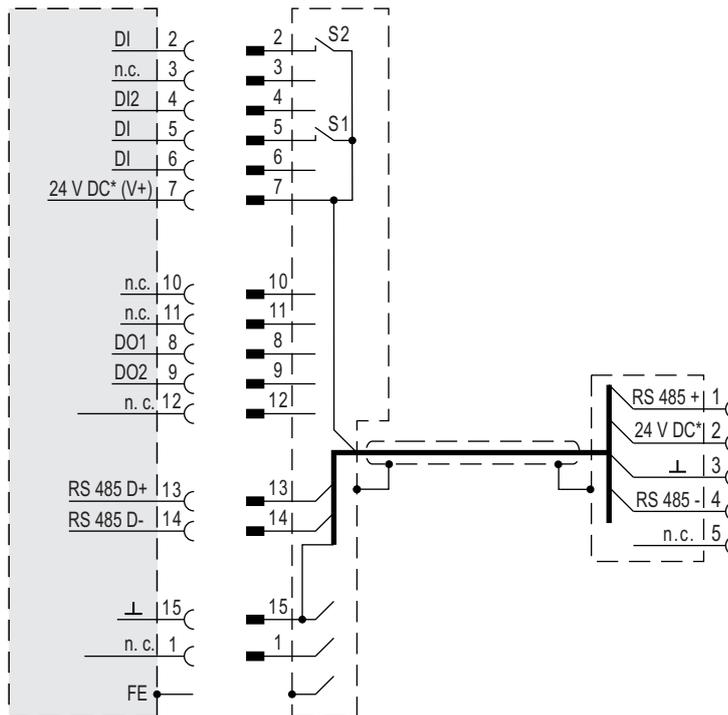
Fig. 12: Connection diagram of 15-pin "remote" connection
