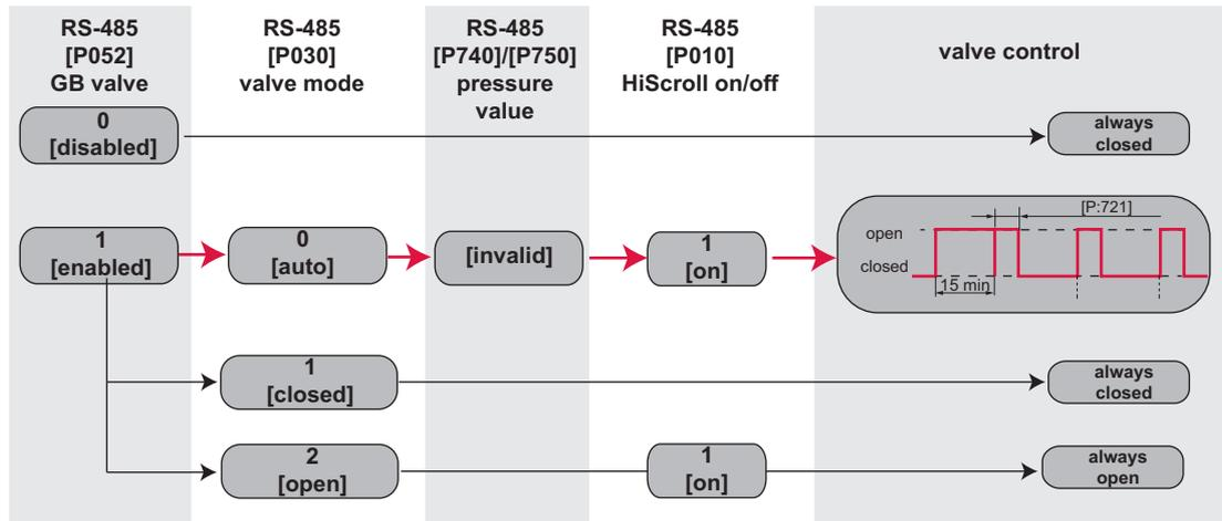
Fig. 19: Gas ballast valve control in automatic mode
