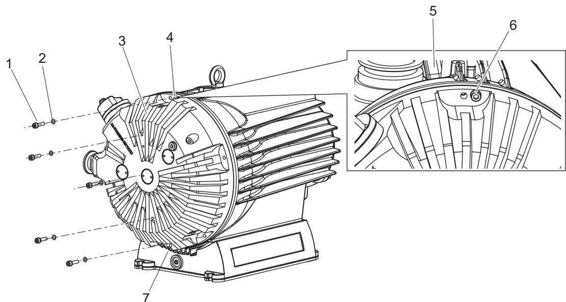
**Fig. 24: Removing the scroll pump spiral housing**
