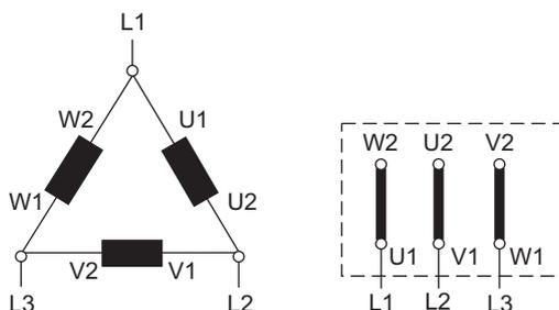
**Fig. 10: Delta connection for low voltage**
