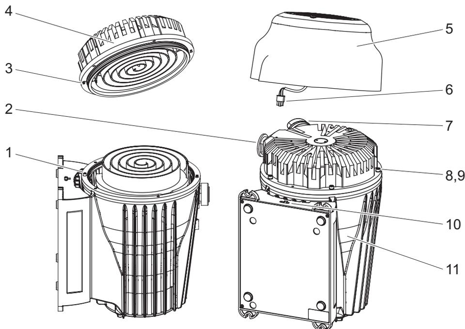
**Fig. 27: Assembling the housing parts**
