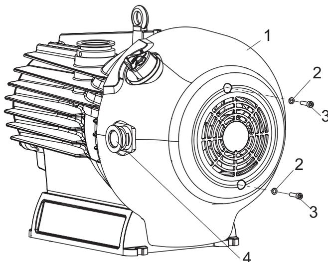
**Fig. 22: Loosening the fan cover on the scroll pump**
