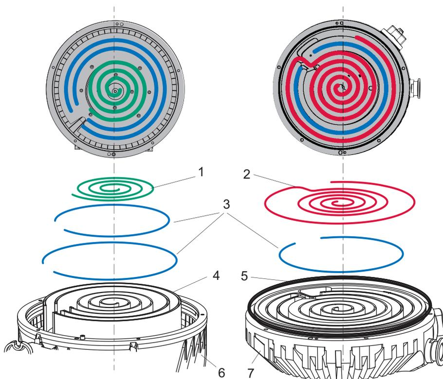
**Fig. 25: Replacing tip seals on scroll pump**
