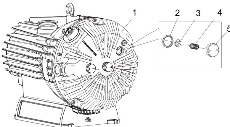
**Fig. 16: Disassembling valves**
