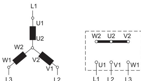
**Fig. 9: Star circuit for high voltage (factory setting)**
