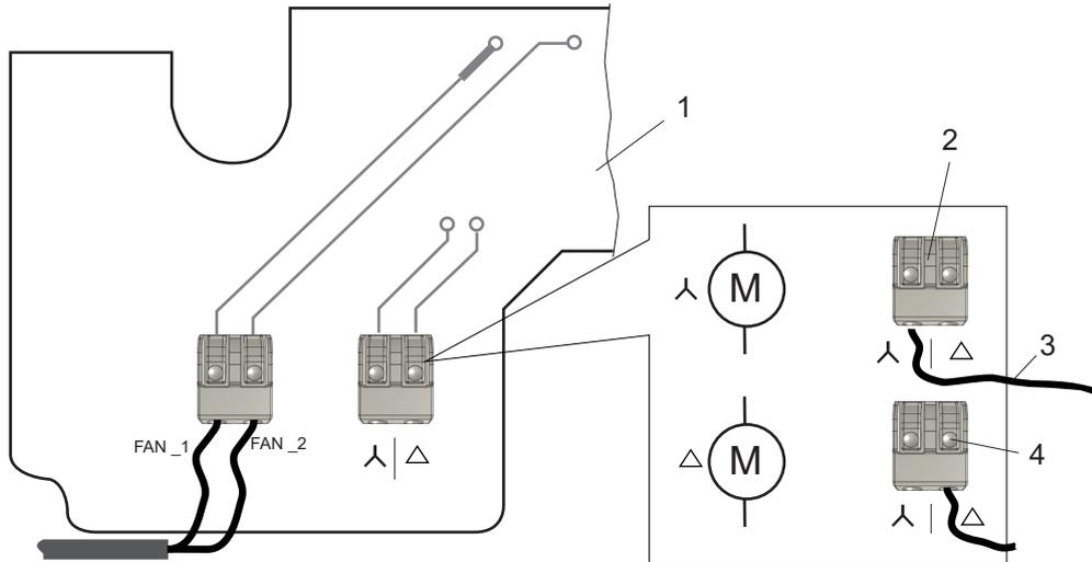
**Fig. 11: Clamping fan connecting cable onto circuit board**
