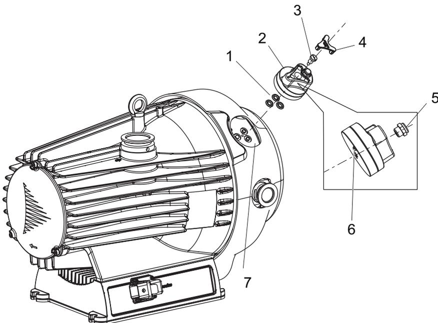
**Fig. 21: Assembling gas ballast valve**
