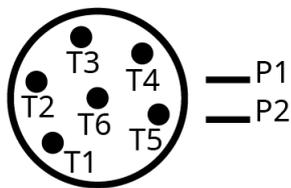
Connection of motor temperature switch (recommended):
