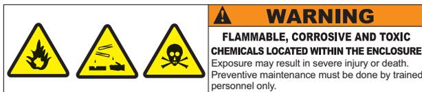
This label warns users about pumped process gases that can be dangerous or toxic and lead to severe injury or death. It specifies that only trained personnel should perform preventive maintenance operations.
