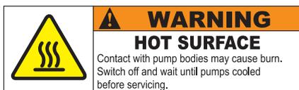
This label warns users that they risk being injured if their hands come into contact with a hot surface: protective gloves must be worn at all times when working on the pump.
